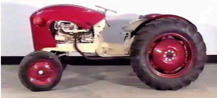
Above Prototype of the tractors designed to utilizes the industrial version of the Holden 132 “Grey Motor” . Acknowledgement Wiki.
