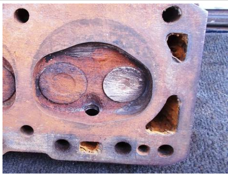
Above Bathtub chamber of standard Red motor head would not give high enough compression ratio for Diesel operation . Pic Warwick
